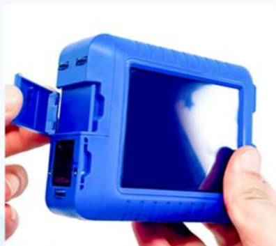
Remove the protective cover
